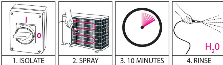
Each Condenser Cleaner Gel pouch is designed to make 8L of usable product. The easiest way to do this is to pour the entire gel pouch into the bottom of our HydroSprayer and then fill with water up to the 8L mark. Alternatively, the product can be mixed in smaller volumes, using 1 part product to 15 parts water. Once the water is added, the product will be ready to use in 5 minutes.
